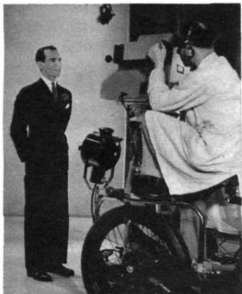
'Tracking up' on Dr. Malcolm Sargent in the studio. The Emitron camera is mounted on a rubber-tyred truck so that it can be moved for close-ups or long-shots.
